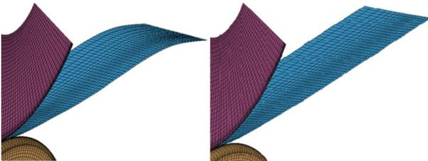
Waves can occur in case guiding is not selected while simulating thin sheet. In reality, this is normal when the coil end is reached. It however has interfering influence on the simulation result. A switch is provided to prevent oscillation.
