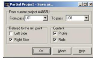
The function **Partial Project Save as** is useful if a certain part of a project, e.g. the left or right side only, the passes only without rolls, or a subset of the passes should be saved to a file. This can be used for combining a new project from already existing modules by the function **Partial Project Add On**.
