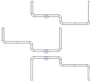
**Modify Start Element, for optimizing the orientation of the profile in the machine, also for changing the opening direction.**
