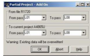
By using the function **Partial Project Add On** you can add such a partial project to your currently opened project. During this operation it is essential that the objects of the added project overwrite the objects of the current project
