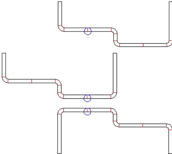
The new function **Modify Start Element** enables defining the orientation of the profile in the machine.
