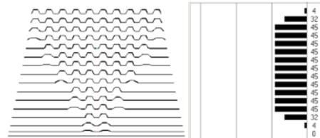
The roll forming process always starts with the inner trapezoids. This is why the material should be able to "flow" to the inside during bending. The user can select if the entire trapezoid or the trapezoid's flank should be formed simultaneously.
