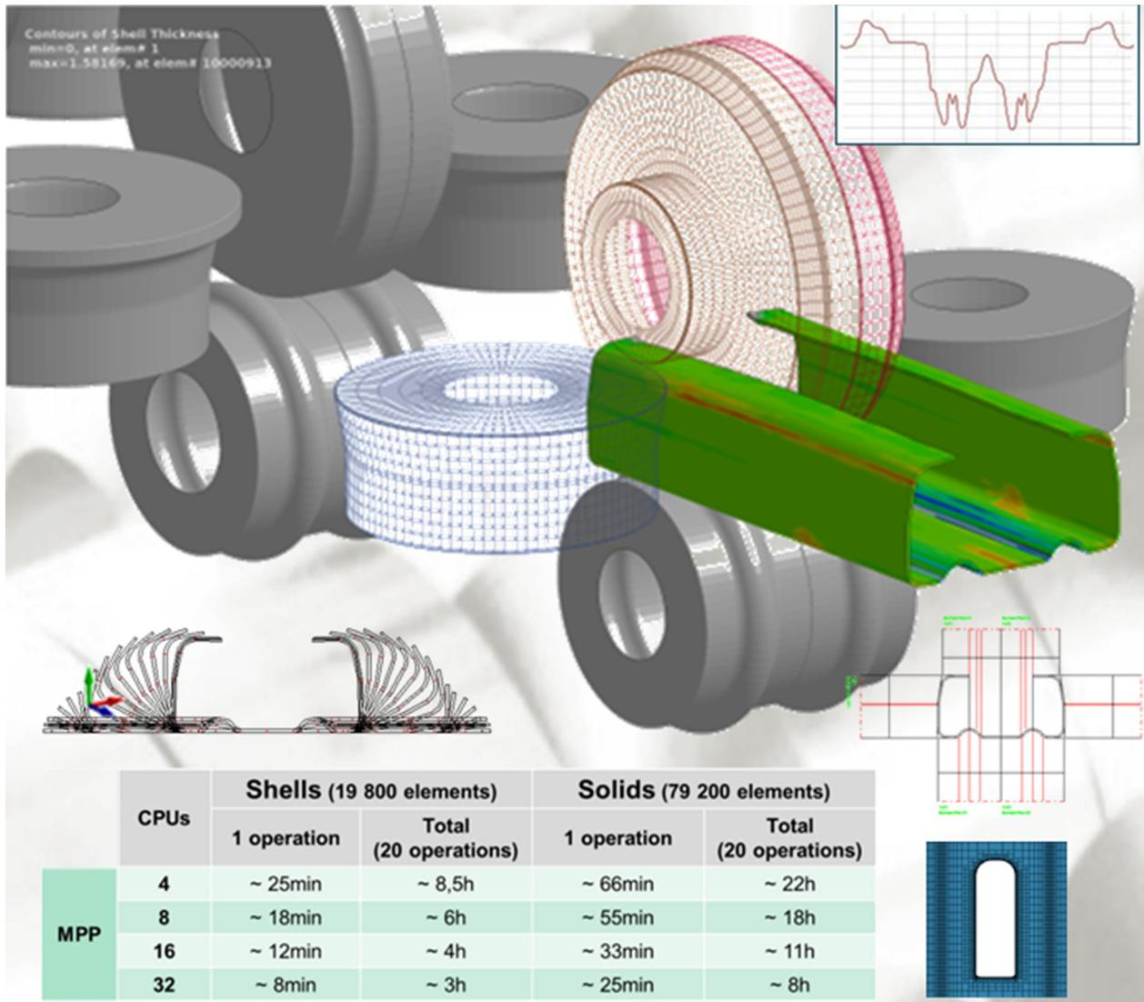
The FEA (Finite Element Analysis) simulation needs amazing short computation time if the proper measures are taken
