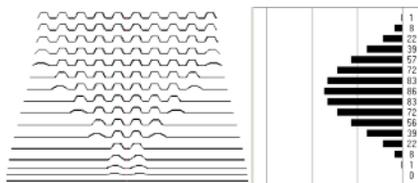
The **cosine band edge course** (left) creates a sine course of the stress of band edge (right). The advantage of this method is the very smooth transition both from the entering flat sheet and to the ready product leaving the machine.
