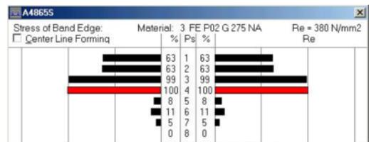
red bar warns about danger: the stress is going to exceed the yield point. While optimizing the flower pattern, the bar diagram is updated simultaneously. Designers like this methods, as they are enabled to check the relative stress while modifying the bend angles.
