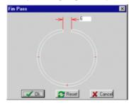
Simply enter the fin width, the tube is bent open automatically to the given width.
