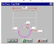
Simply enter the roll width, the fin height, the fillet radii and the air gap between top and bottom roll. The roll is created automatically.
