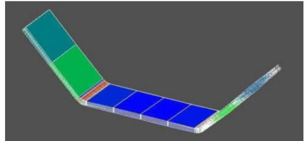
Running of a flat sheet into a stand with 45 degree rolls was simulated. Without clearance angles considerable strain is shown in the legs (green: medium strain).
